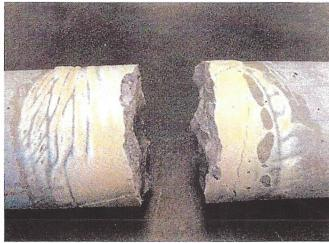
The axial alignment and loading method is taken from ASTM C633, which is used to determine the adhesion or cohesion strengths of coatings to substrates. The test was conducted at a loading rate of 0.05 in./min of cross head travel. The photograph to the right shows the break occurring through one of the two concrete cylinders, and not at the bonding line of the epoxy.
